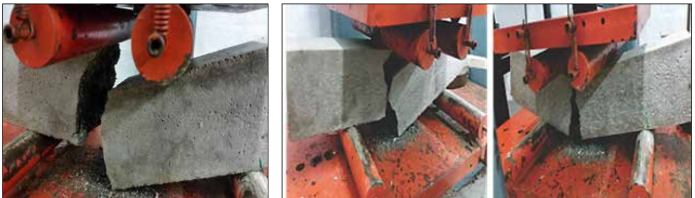
Figure 16. Flexural mode and pattern of failure for (a) CTRL, (b) NonC, (c) N-treated NSFRC beams
