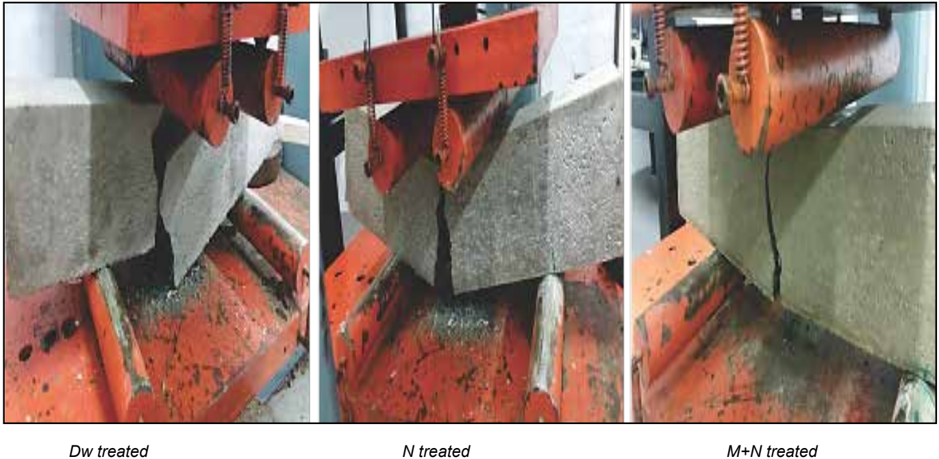
Figure 12. Deformation of tested NSF reinforced concrete beams
