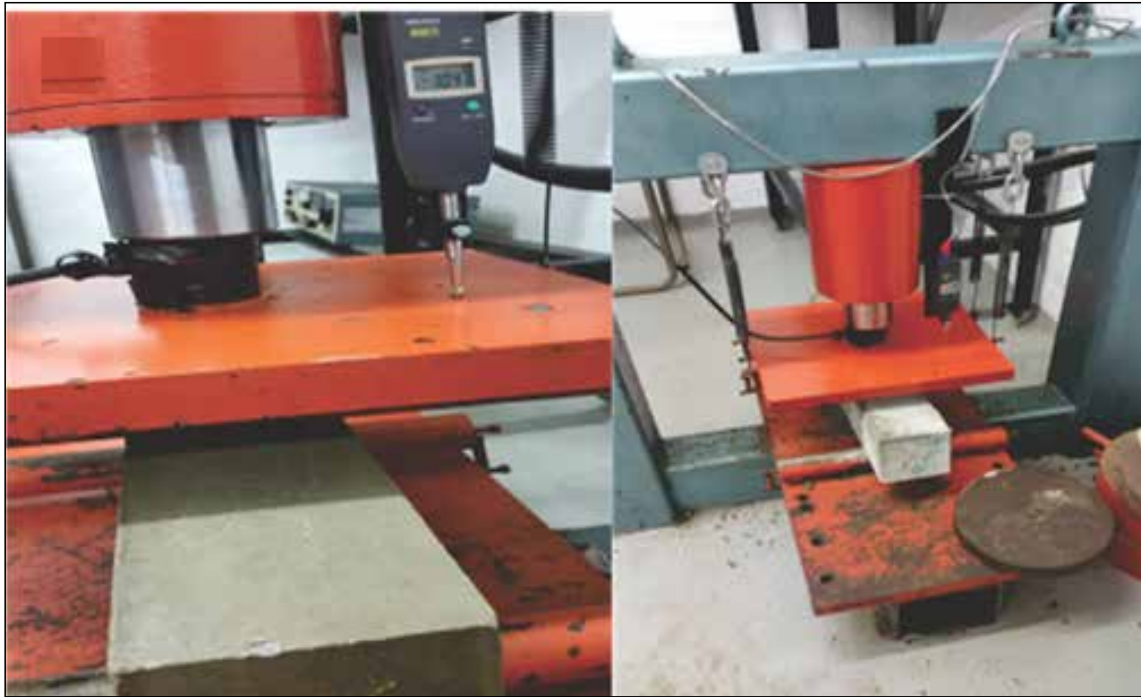
Figure 4. Test setup for beam of NSFC
