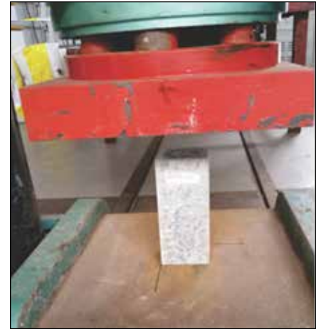
Axial compression testing
